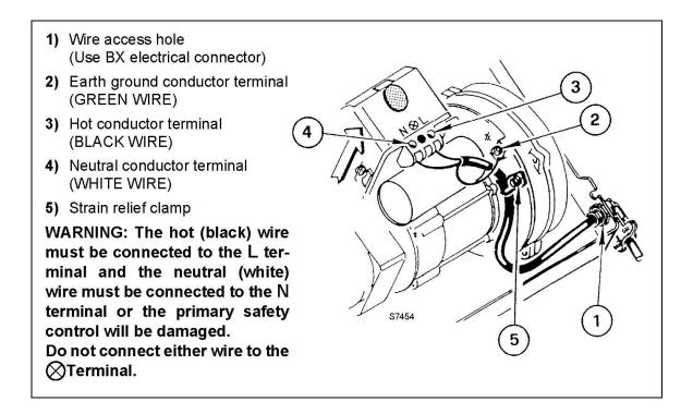
The burner may be controlled using either a DIRECT LINE VOLTAGE control circuit (120V AC 60 cycle) **OR** a LOW VOLTAGE control (24V AC 60 cycle) using a R8038A Honeywell switching relay or equivalent.
