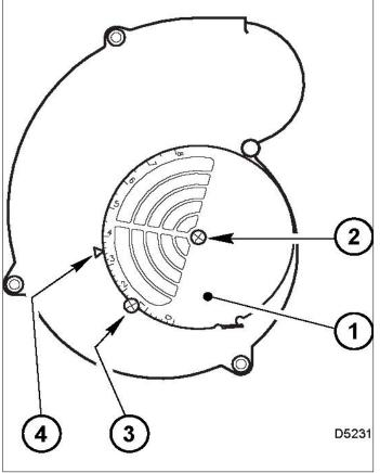
adjustment plate will vary on each installation. Use instruments to establish the proper settings for maximum CO<sub>2</sub> and a smoke reading of zero.
