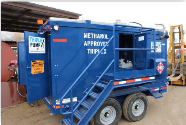
External stairs provide safe easy access to the roof mounted product tank
