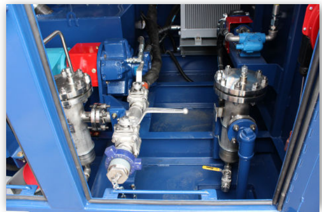
Sump pump and remote fluid supply connection provide versatility
