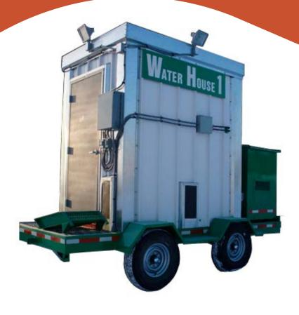
The ESI Water House is designed to keep open ice holes over bodies of water where explosive gases may accumulate. With safety and practicality in mind, our unit is designed with two separate compartments; one implementing explosion-proof components, the other housing the generator or other electrical devices.
